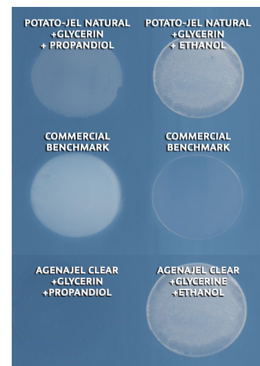
Fig. 6. Dried thickener starch films to show transparency
